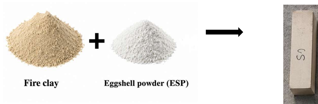
Fig 1: Raw materials and preparation process of fire clay–ESP brick specimen
