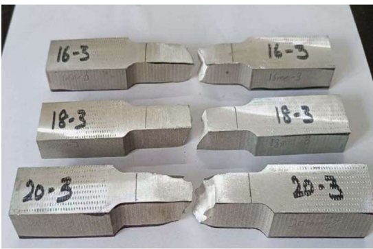
T8 Tensile Specimen After Failure
