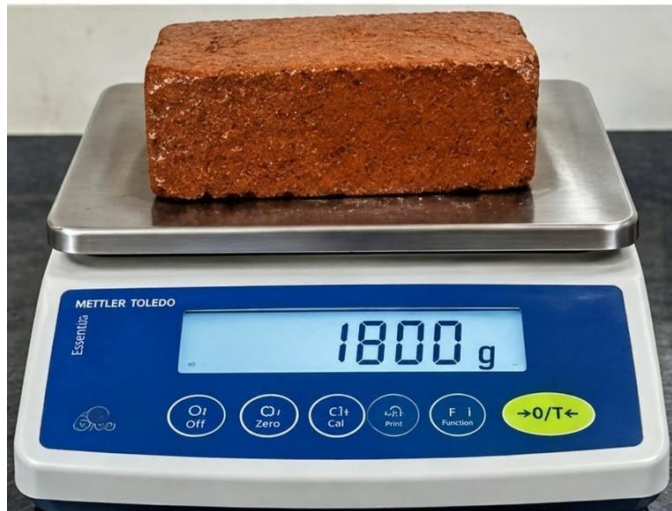
Fig.3. Density test in clay brick
