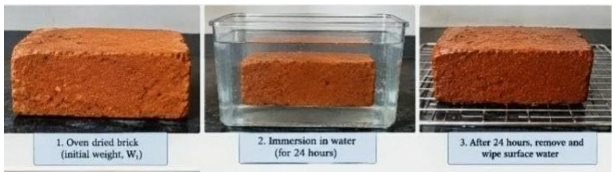
Fig.5. Water absorption test in clay brick
