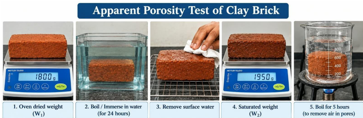
Fig.6. Apparent porosity test in clay brick
