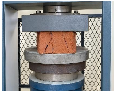
Fig.4. Compressive strength test in clay brick
